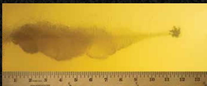
Gold Dot has been proven to provide optimum penetration and expansion through ballistic gelatin and all barriers used in FBI protocol testing. Tests conducted with 9mm Luger 124-grain +P Gold Dot (23617).
