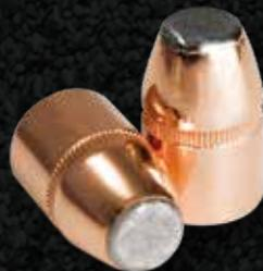
Speer® electrochemically bonds the DeepCurl jacket to the lead core to create the toughest, most accurate handgun hunting bullet possible. Pre-formed petals expand reliably and consistently and the bullet's high weight retention ensures deep penetration on heavy-bodied game.
